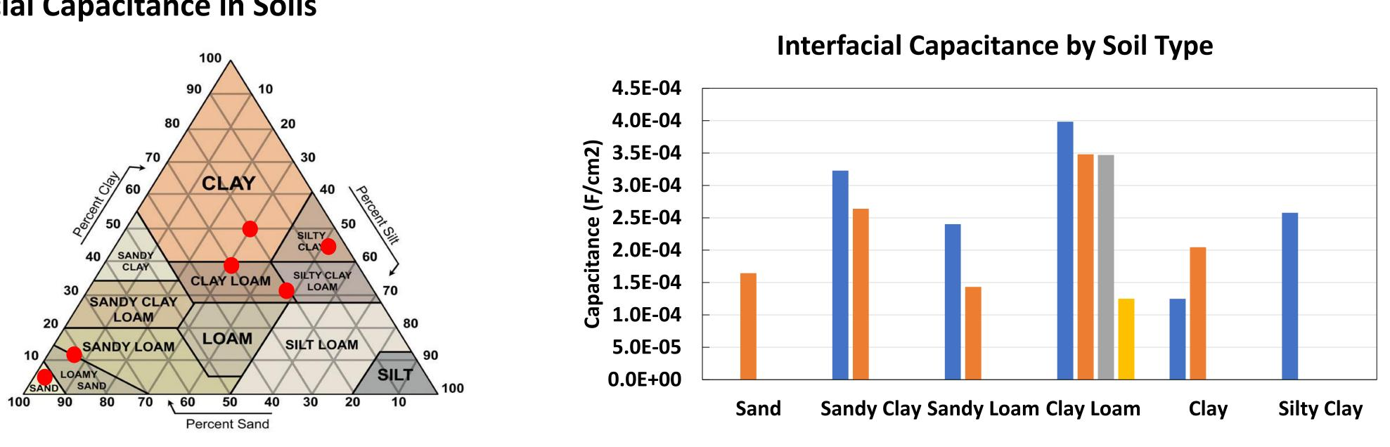
USDA soil texture triangle classifying soil types according to percentage of sand, silt, or clay content (<2mm = Sand, <50μm = silt, <2μm = clay). Red dots indicate soil compositions tested.
